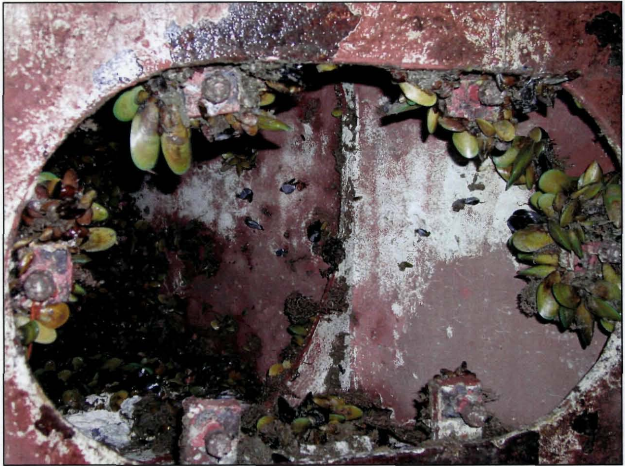
Plate 1.3: The sea chests of the Alexander Slobodchikov , cleaned in the Lyttelton dry-dock, contained large clumps of greenshell mussels ( Perna sp.). Viable errant polychaetes and motile crustaceans and molluscs were common within these clumps. This picture was taken after approximately 90 % of the mussels had already been removed from the sea chest. Photo: O. Floerl, NIWA.
