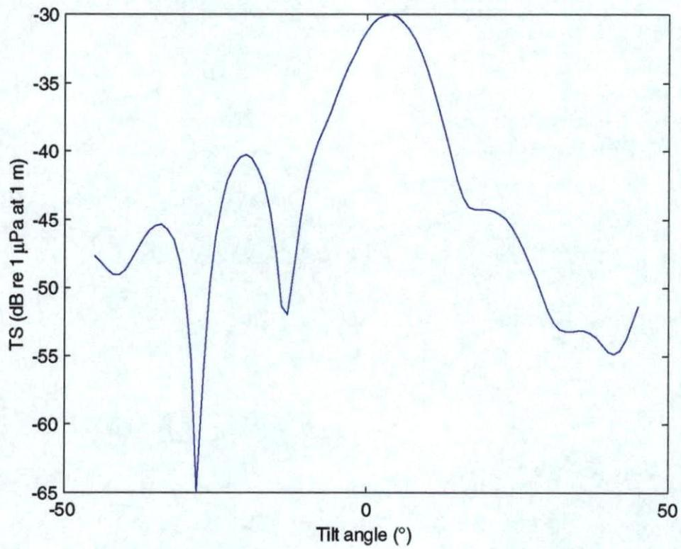
**Figure 6: An example of the TS/tilt relationship obtained from the hake swimbladder modelling. Positive tilt angles correspond to a fish head up attitude.**
