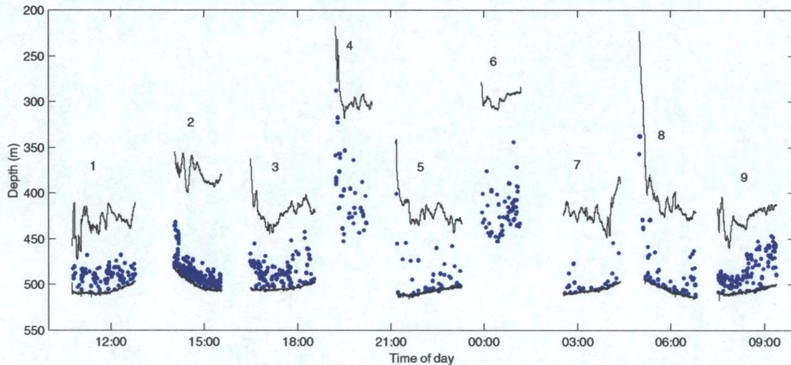
Figure 2: Vertical distribution of single target echoes from the 38 kHz towed echosounder. The upper set of lines is the depth of the echosounder, and the lower set of lines is the bottom. Single target echoes are indicated by the dots. The gaps in the data are a result of turns at the end of each transect. The numbers correspond to transects.
