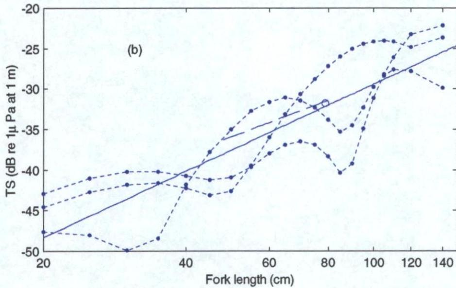
Figure 5: The target strength/fork length data obtained from swimbladder modelling and *in situ* data. The dashed curves and dots are from scaled swimbladders. The dashed line is from Lillo (1996), and the circle is the *in situ* point. The solid lines are regressions fitted to the swimbladder and *in situ* data. Part (a) contains results for 12 kHz, and (b) contains results for 38 kHz.
