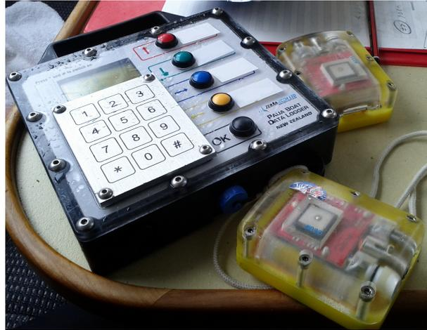
**Figure 1: Boat unit and two turtle units, photographed after the data upload process, during the fishdown experiment.**
