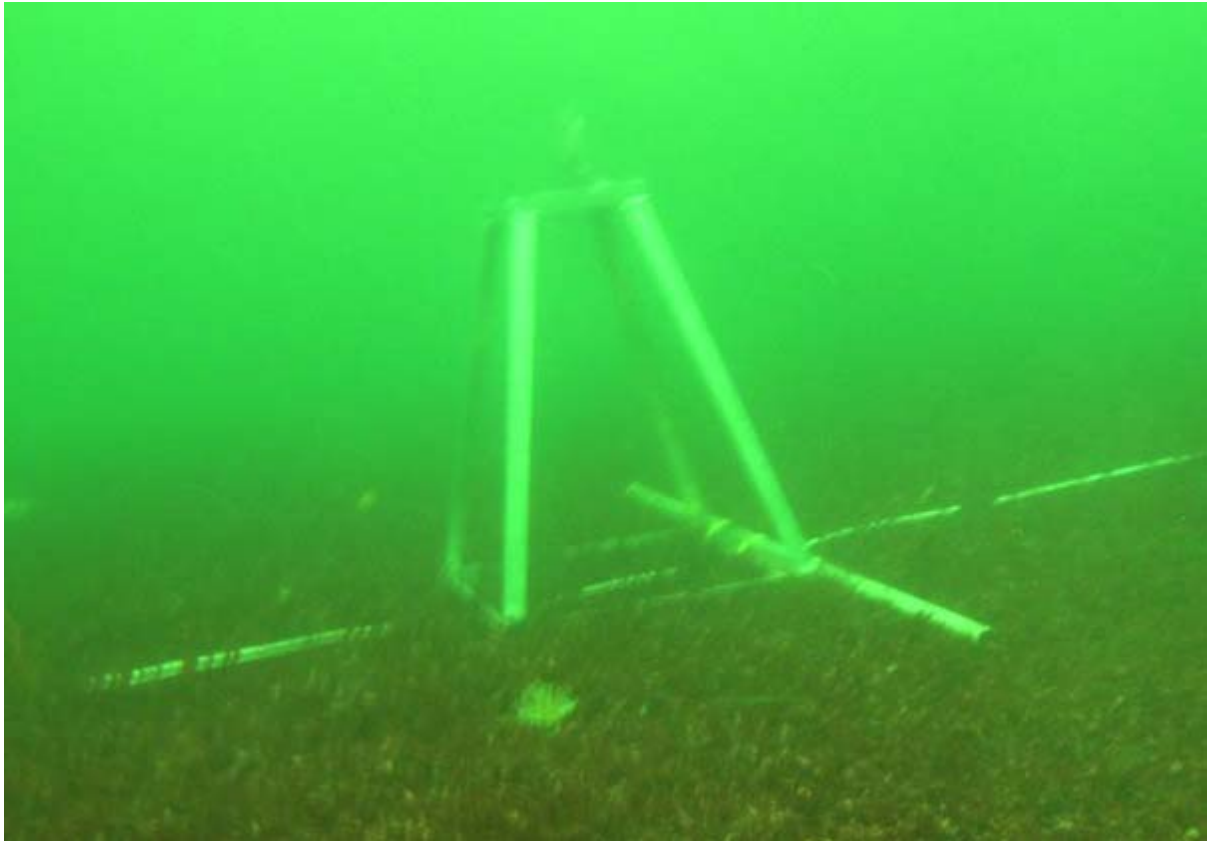
Figure 4: Photo-quadrate ( 0.25 \text{ m}^2 ) camera and frame with 2 m pole on transect line. All scallops within the 2 m pole length were collected and measured.
