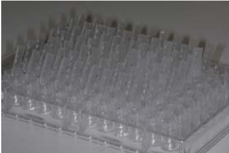
Cleaned wafers stored in a tray prior to mounting on glass slides.
