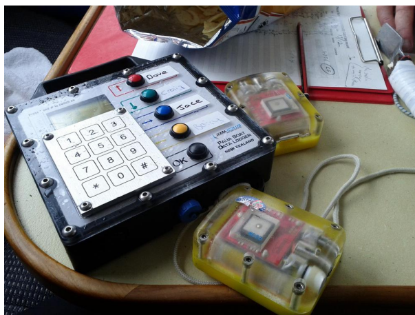
Figure 1: Pāua ( Haliotis iris ) dive loggers consisting of a larger boat unit (with buttons for recording catch bags and a key pad for entering catch weight and other data) and "turtle loggers" carried by divers.
