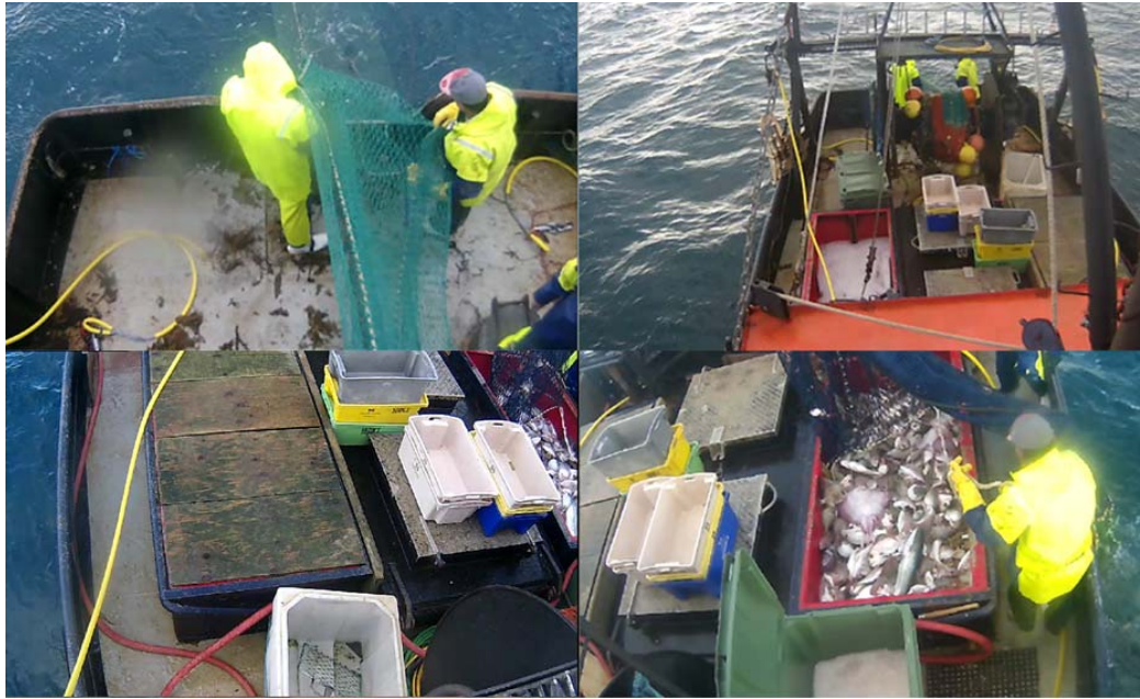
Figure 2: Example of the first general camera configuration used. Clockwise from top left: view of the trawl net coming in on the stern; deck overview; starboard catch sorting and discard control point area; and port catch sorting and discard control point areas. The fourth camera was used to provide a close up view of the port slurry bin in case it was used to sort catch.
