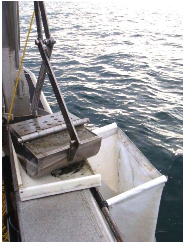
Figure 17: Van-Veen grab full of sediment before samples had been retrieved.
