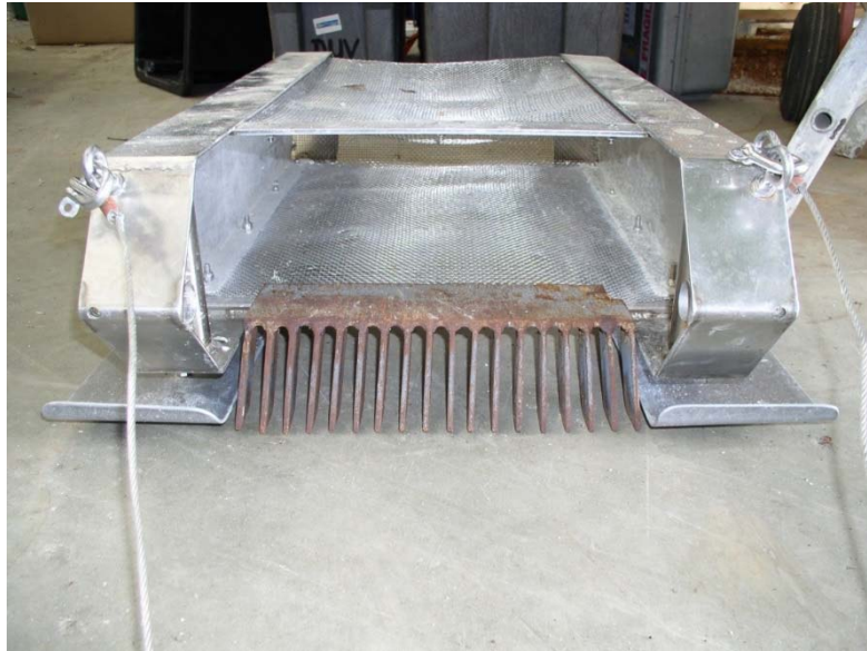
Figure 16. Modified epi-benthic sled showing wider skids and steel tines designed to pick up large (over 10 mm) organisms living at the surface of the sediments.
