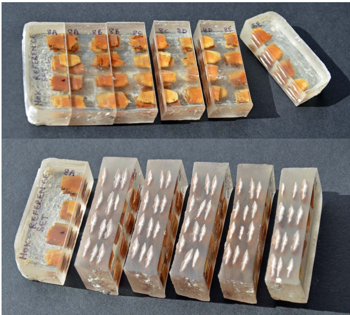
Figure 3: Resin block (block #8 of the hoki reference set), comprising six sub-blocks, holding 60 cross-sectioned baked otoliths in five groups of 12.
