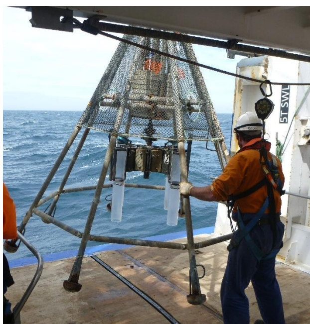
Figure 6: Ocean Instruments MC-800 multicorer deployment from RV Tangaroa during TAN1701.
