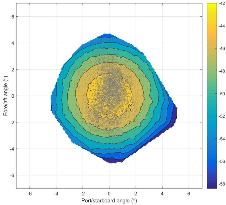
**Figure A1:** The estimated beam pattern from the sphere echo strength and position for the 38 kHz calibration. The '+' symbols indicate where sphere echoes were received. The colours indicate the received sphere echo strength in dB re 1 m<sup>2</sup>.
