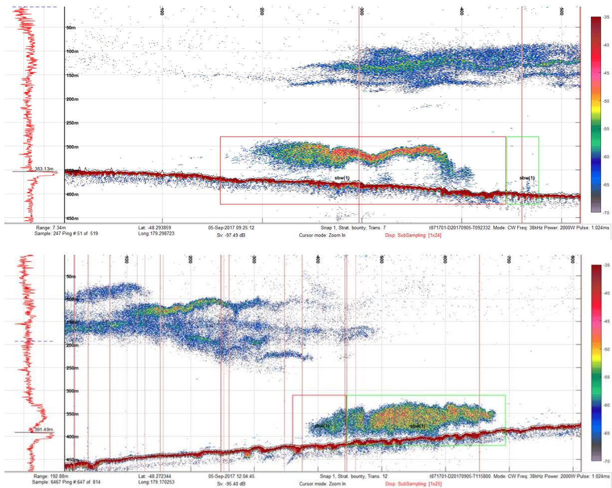
**Figure 4: Example of acoustic echogram collected at the Bounty Plateau during snapshot 1 on 5 September 2017 on transect 7 (upper panel) and transect 12 (lower panel). Red vertical lines are where ping drop-outs due to bubble aeration in poor weather were removed. Southern blue whiting aggregations were defined inside a rectangular box.**
