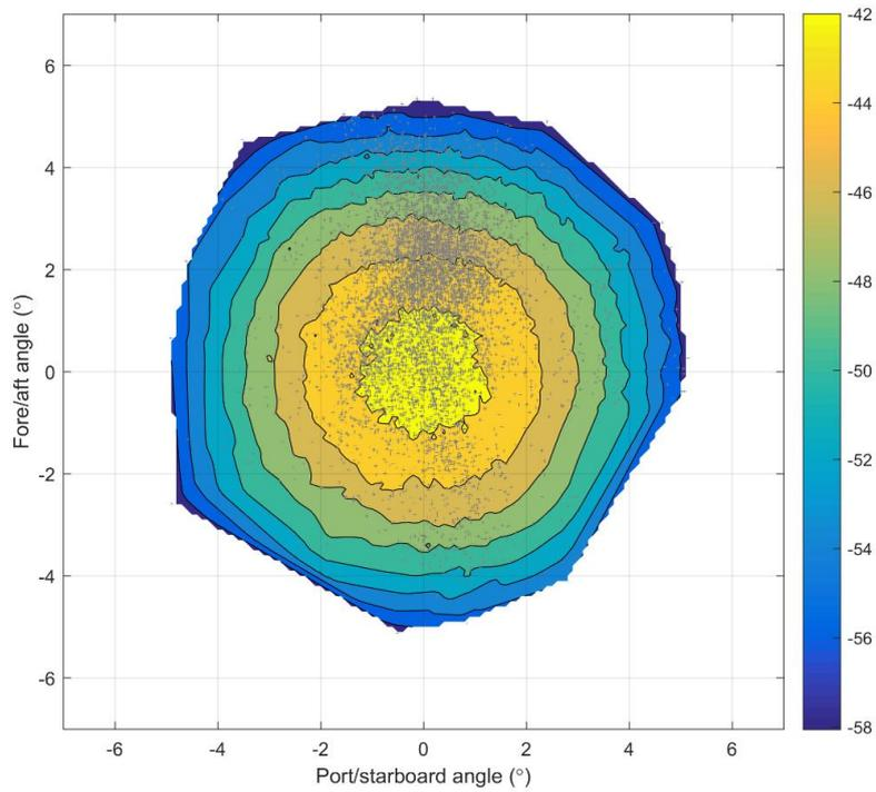
**Figure A3:** The estimated beam pattern from the sphere echo strength and position for the 70 kHz calibration. The '+' symbols indicate where sphere echoes were received. The colours indicate the received sphere echo strength in dB re 1 m<sup>2</sup>.
