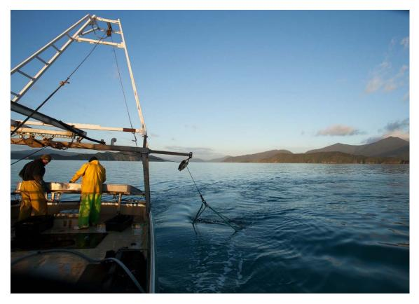
Figure 4: Stern of FV *Okarito* showing deployment of ring-bag dredge in Marlborough Sounds. Photo credit: J. Williams.
