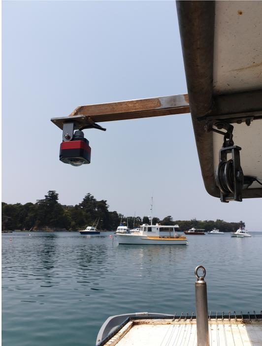
(a) Full hemisphere cameras deployed on an extendable boom out from the vessel haul station.
