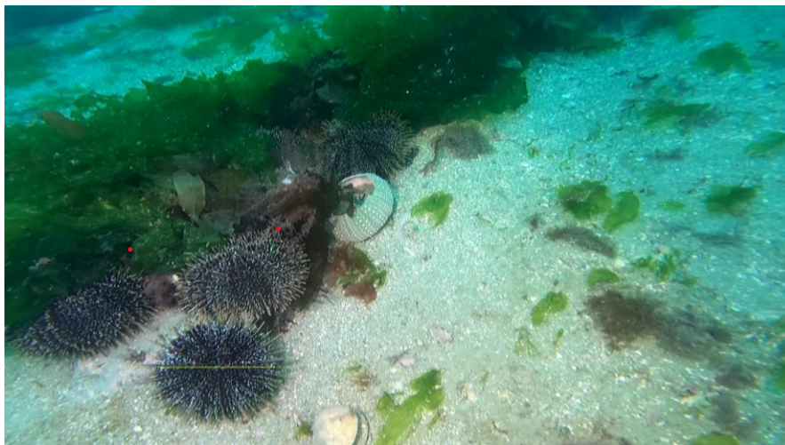
Figure 5: Image processing for measurement of kina test diameter. A (yellow) line is drawn using Fiji ImageJ software and the scaling lasers (red dots) used to convert the line length to an estimated test diameter.
